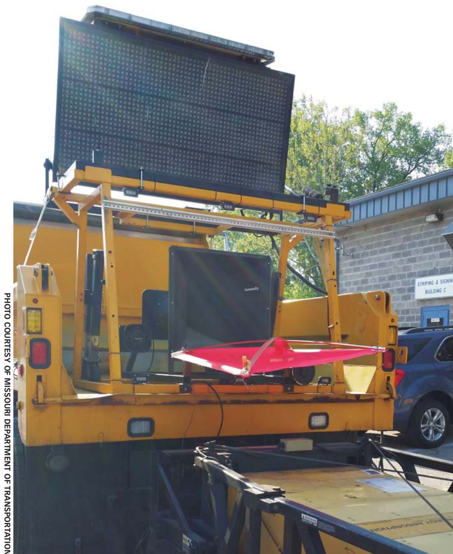
A speaker for an alarm device mounted on a VMA.
